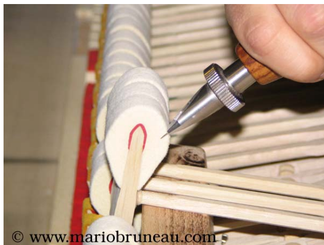
A voicing tool used to harmonize the piano by means of voicing the hammer heads
